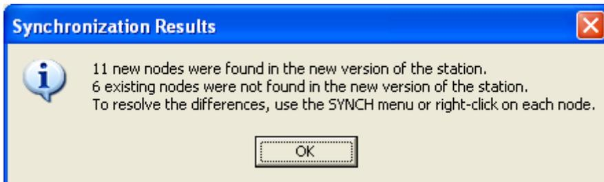
The station tree will then be updated to reflect these changes. New nodes are displayed in the tree in blue, while missing nodes are shown in red. If the missing nodes had been selected, or if the new nodes were found in a selected container, the names will still appear bold to indicate the selection.
